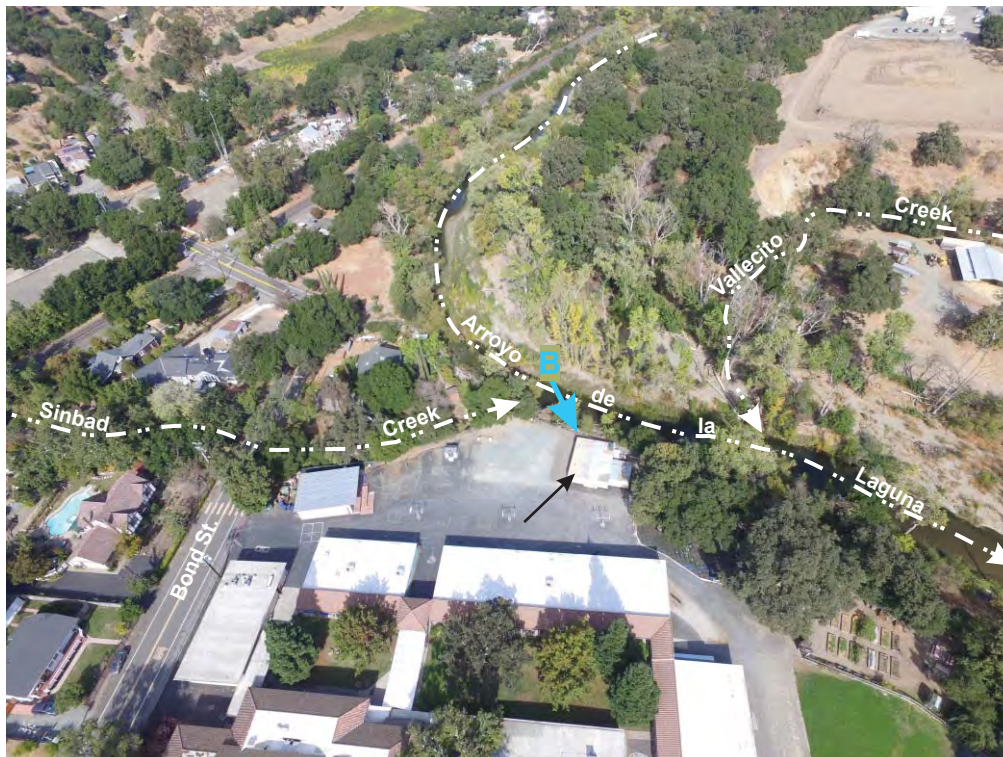
Aerial Drone Image 1. Northerly view across Sunol Glen School. Blue arrow is reported approximate location of Arroyo de la Laguna Creek bank overtopping by flood water on January 1, 2023, due to channel blockage at the bridge crossing downstream. Black arrow points to re-located storage containers.
